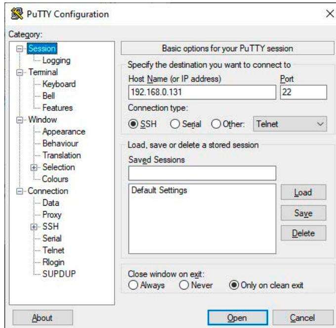
Under **Session** you can enter the IP address of the EW-DX. Choose SSH connection on port 22. For easy reuse, you can save the settings with the **Save** button.
