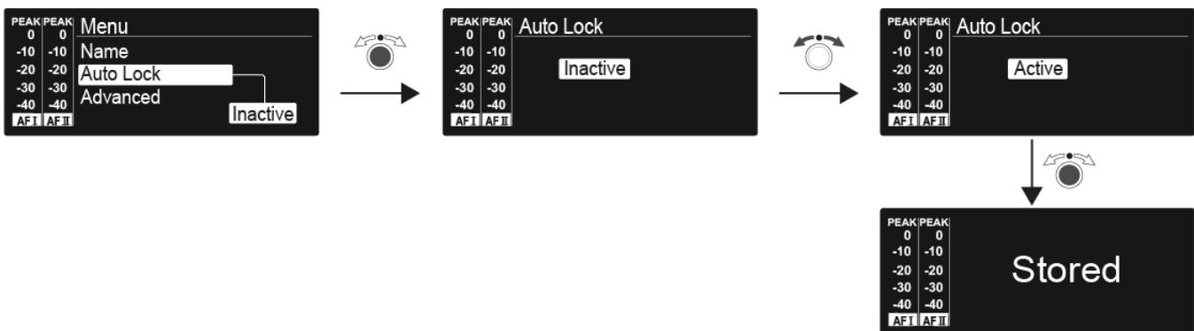
This lock prevents the transmitter from being unintentionally switched off and also prevents any unintentional changes to the transmitter's configuration. In the standard display, the lock icon shows whether the lock-off function is currently switched on.
