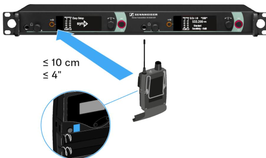
The parameters are transferred to the receiver. The blue LED blinks during transmission.
