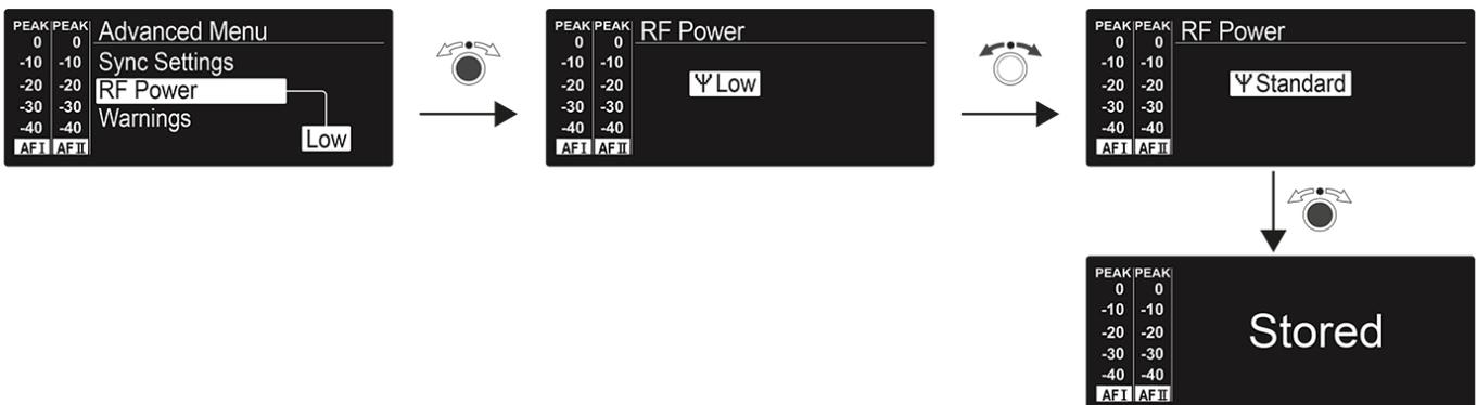
You can configure the transmission power in three steps in the **RF Power** menu item. Please note the general conditions and restrictions for the use of frequencies: [www.sennheiser.com/sifa](http://www.sennheiser.com/sifa)
