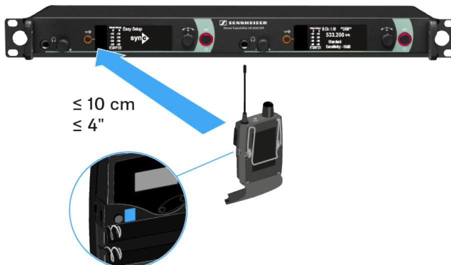
The next unused frequency preset is transferred from the receiver to the transmitter.
