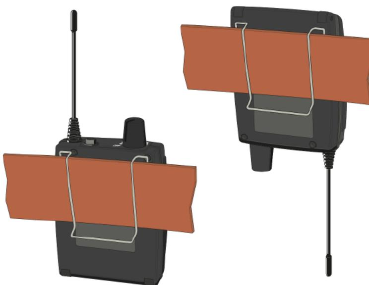
The belt clip is secured so that it cannot slide out of its fixing points accidentally.
