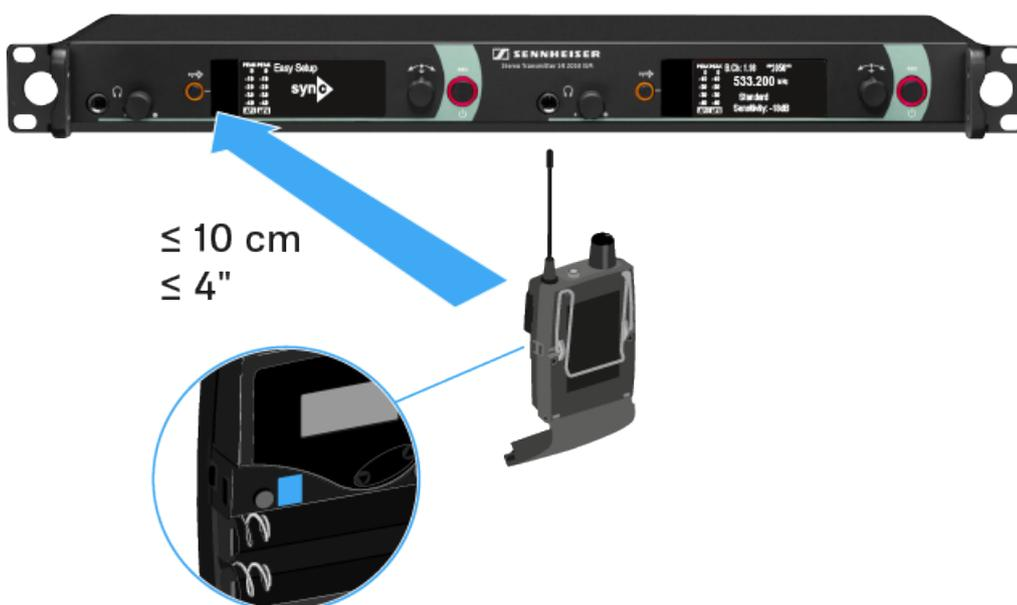
The selected transmitter becomes the master transmitter. The display panels of the other transmitters will display the message **Assign New Frequency?**
